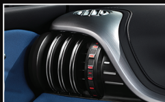
Dumbbell-Style Air Conditioning Vents
